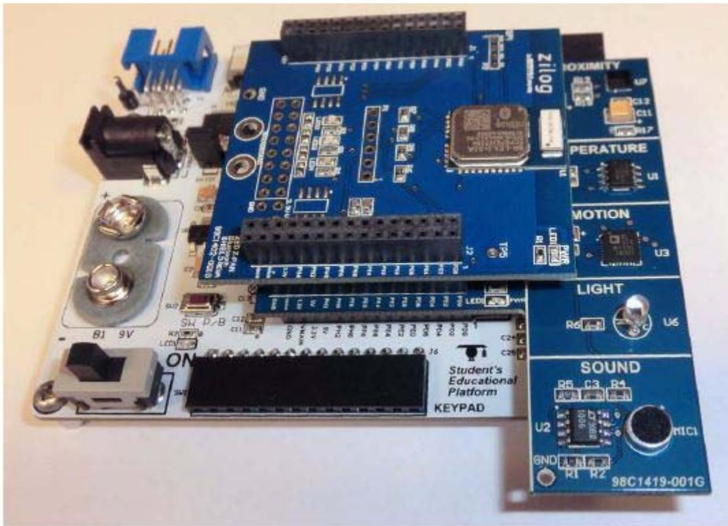
**Figure 14. Shields Stacked onto the ZSED Platform**
