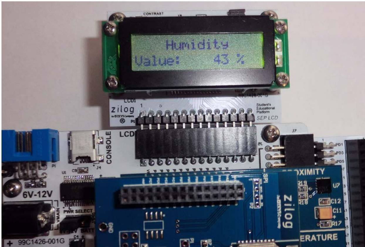
Figure 21. A Humidity Reading on the ZSED Platform's Optional LCD Module
