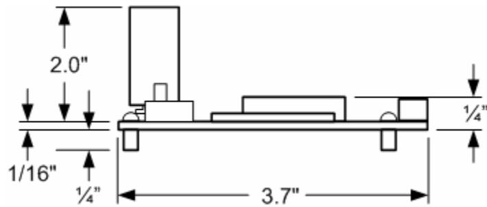
Figure 30. ZSED Platform Side View
