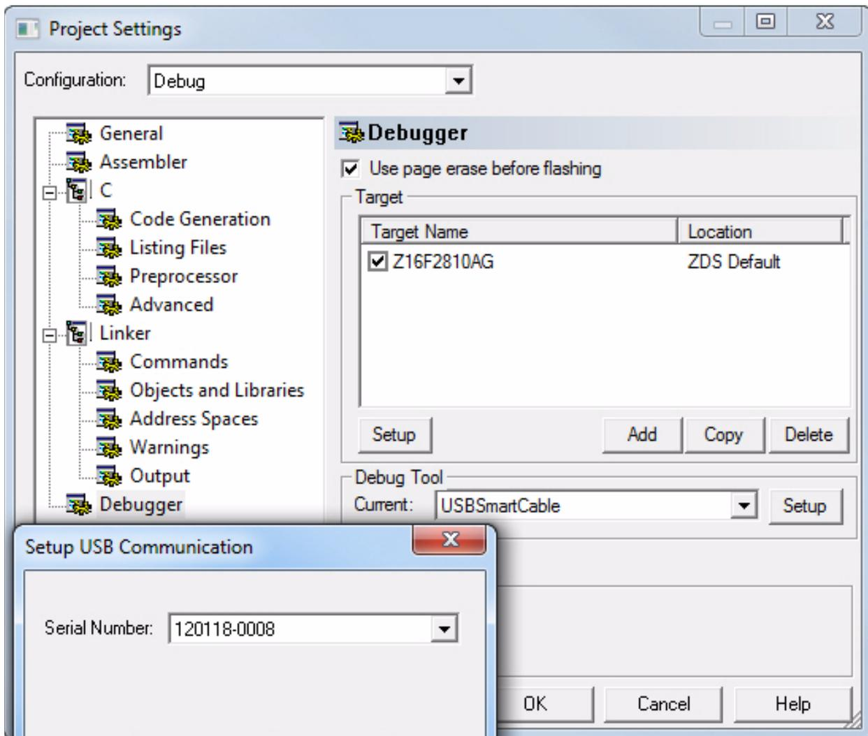
Figure 23. USB SmartCable Serial Number Register
