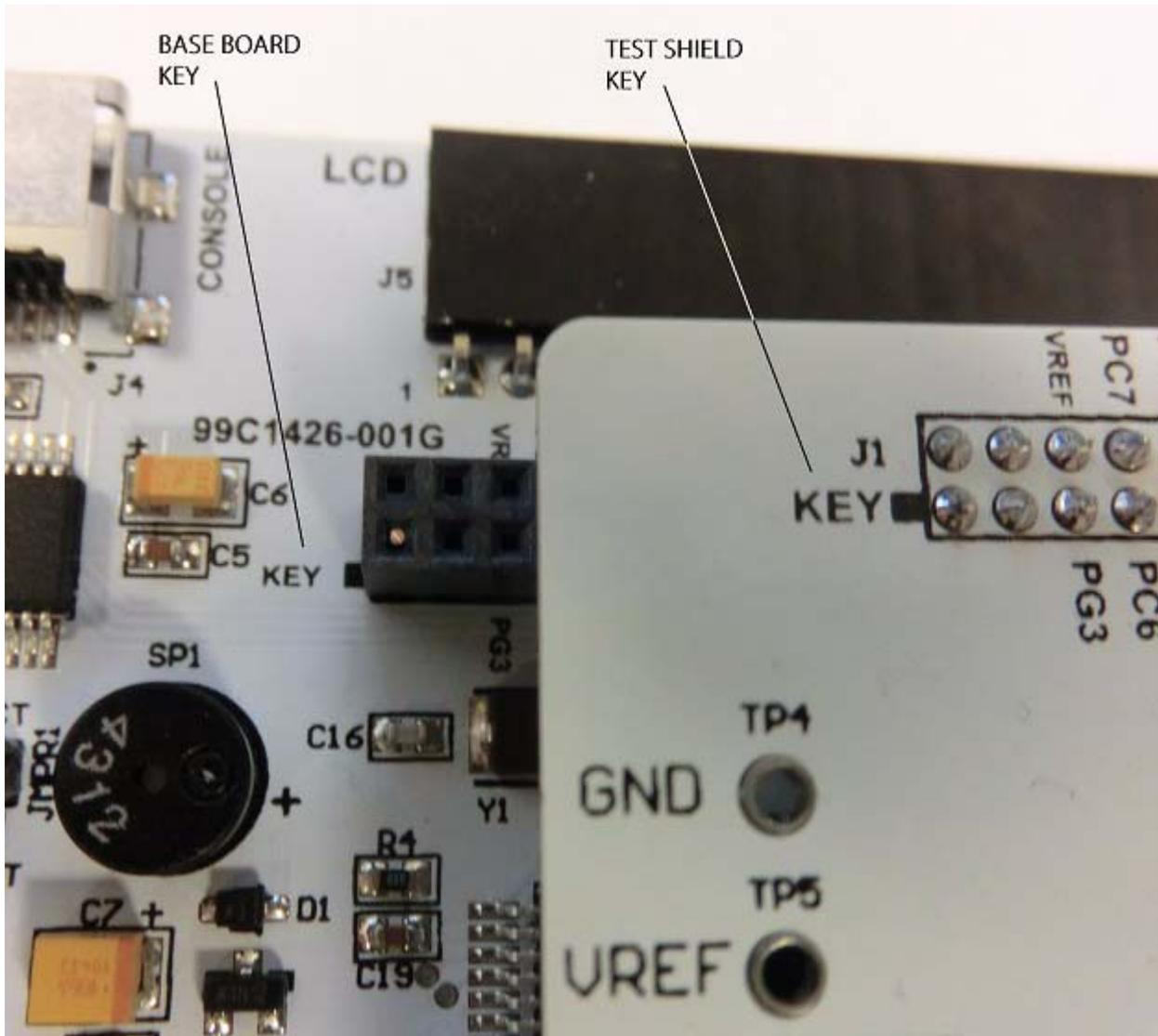
Figure 5. Key Alignment BaseB Shield
