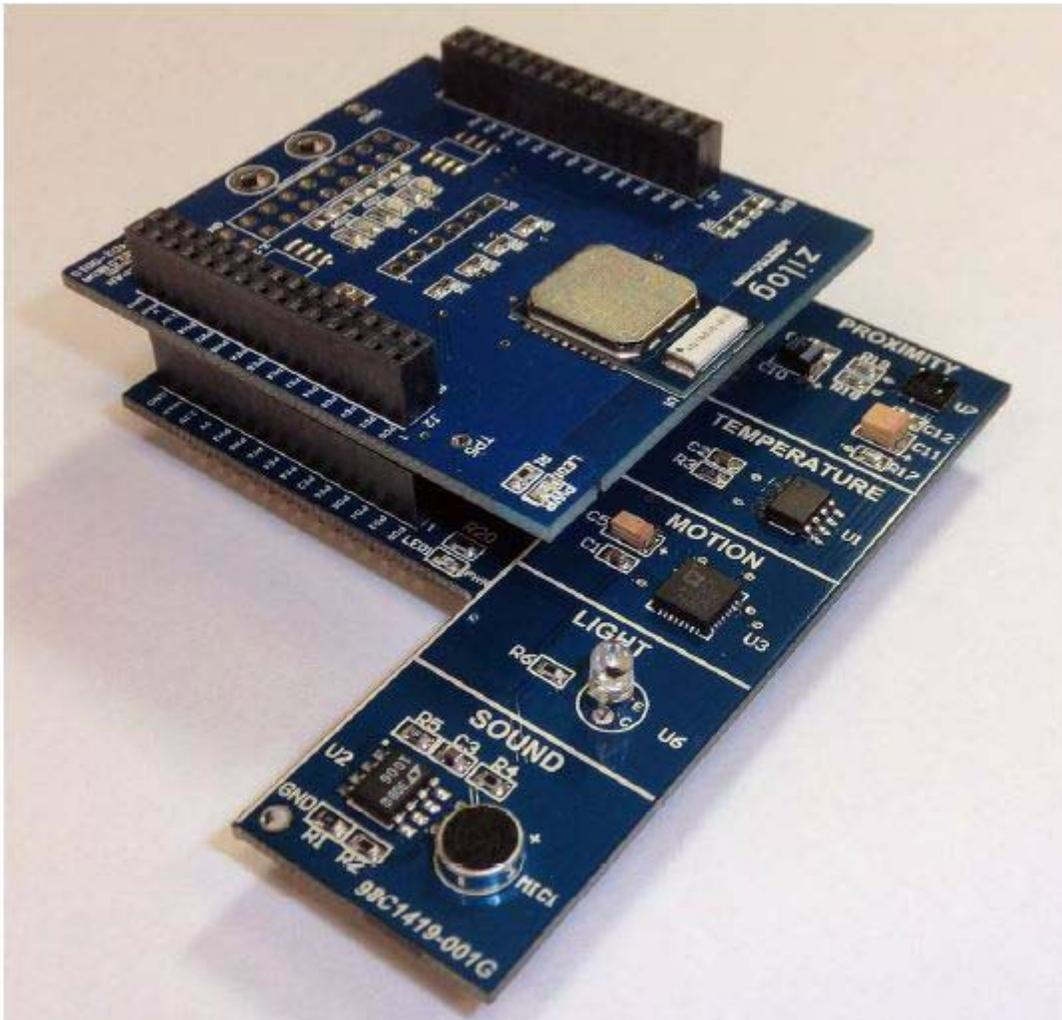
Figure 13. Stacked Bluetooth LE and World of Sensors Shields
