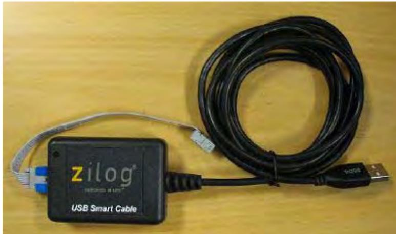
Figure 11. Programming Cable Shown with USB SmartCable Attached
