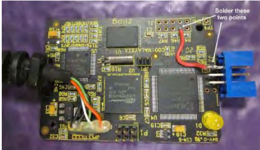
Figure 12. Solder Connections for Modifying the USB SmartCable
