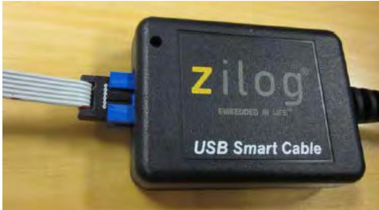
**Figure 8. Completed USB SmartCable Assembly**
