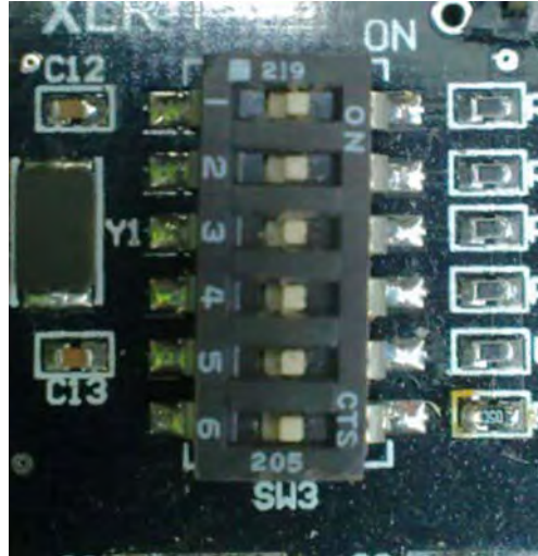
Figure 4. The 6-Position DIP Switch for Setting the DMX512-A Receiver Address
