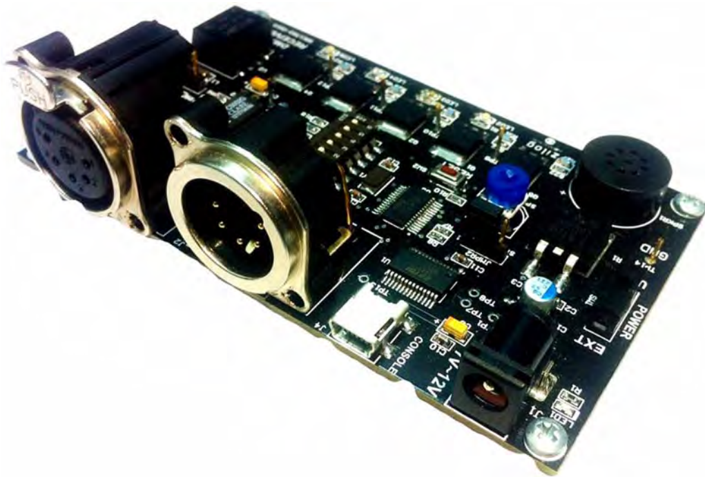
Figure 1. The DMX512-A Receiver Reference Design
