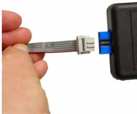
Figure 1. Connecting the Six-Conductor Ribbon Cable to the USB Smart Cable
