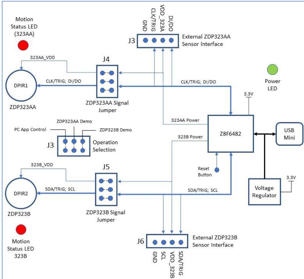
Figure 7 - ZDP323 Digital PIR Evaluation Board Block Diagram
