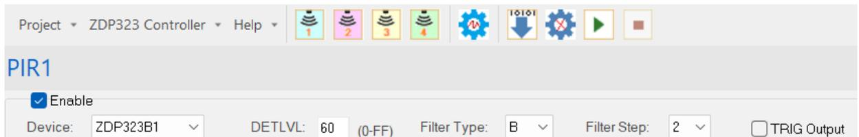
6. Click “Program Device Configurations” to configure the selected device(s) with the parameters.
