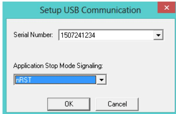
If using nRST for stop mode signaling:
