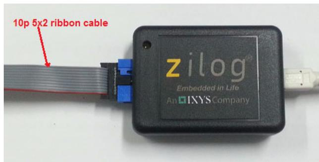
**Figure 3. Connecting the 10-pin Ribbon Cable to the S3 Flash ISP II**
