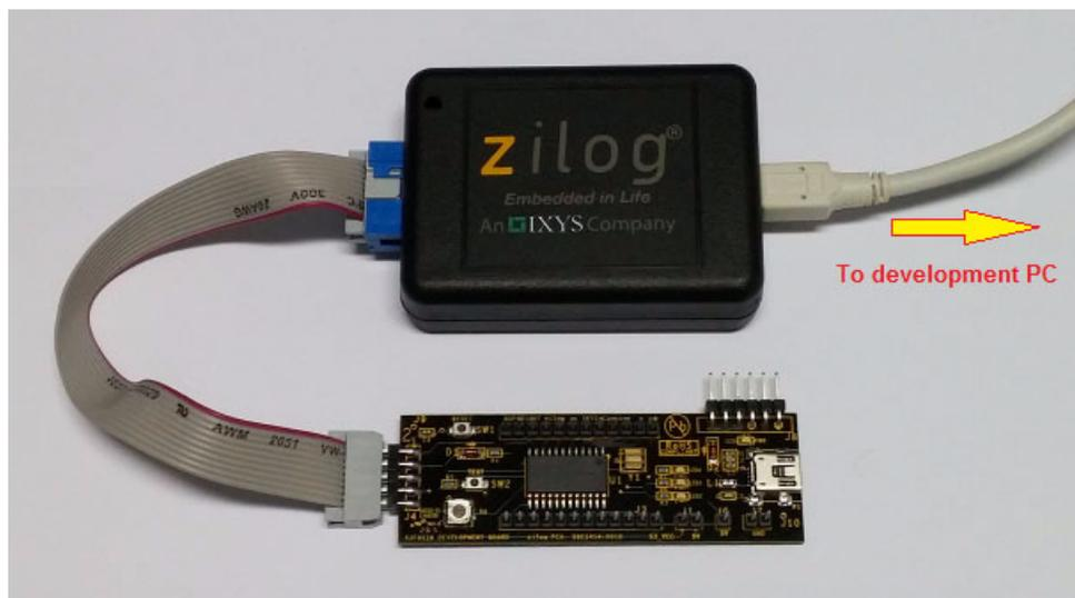
Figure 5. The Completed ISP II and Development Board Assembly
