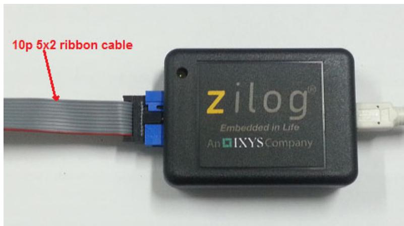
**Figure 3. Connecting the 10-pin Ribbon Cable to the S3 Flash ISP II**
