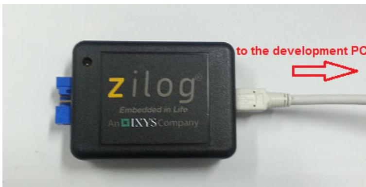
**Figure 2. Connecting the S3 Flash ISP II to the Development PC**
