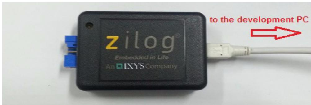
**Figure 2. Connect the S3 Flash ISP II to the Development PC**
