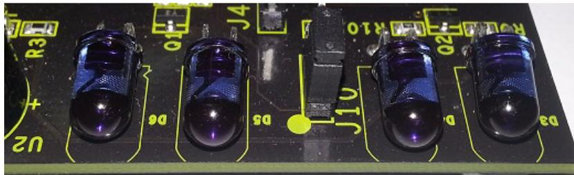
Figure 16. TSAL6200 Infrared Emitting Diodes
