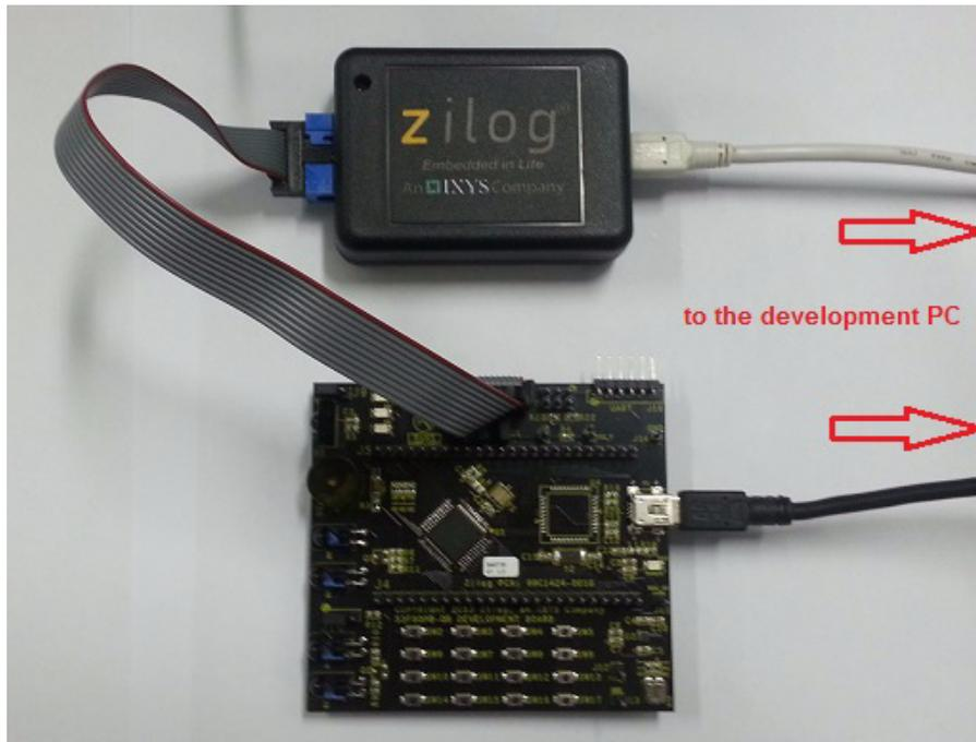
Figure 6. The Completed ISP II and Development Board Assembly
