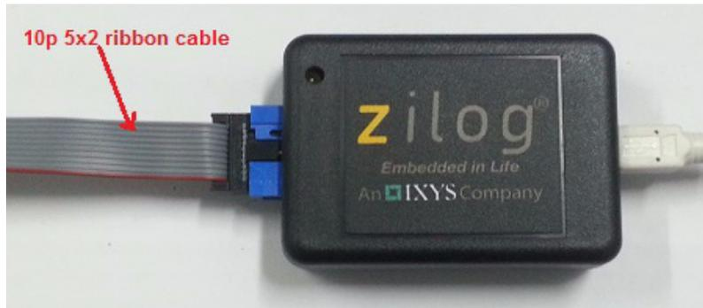
Figure 3. Connect the 10-Pin Ribbon Cable to the S3 Flash ISP II
