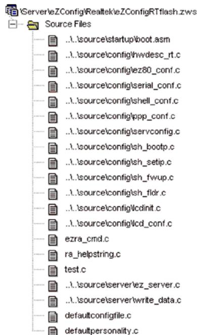
Figure 5. eZConfig Server Project Files for the eZ80L92 Microprocessor
