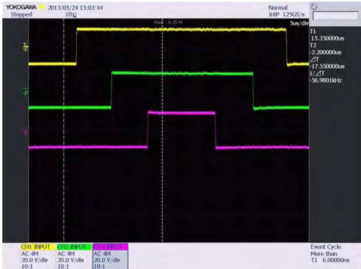
Figure 9. Alternate-Reverse Space Vector Modulation Pattern
