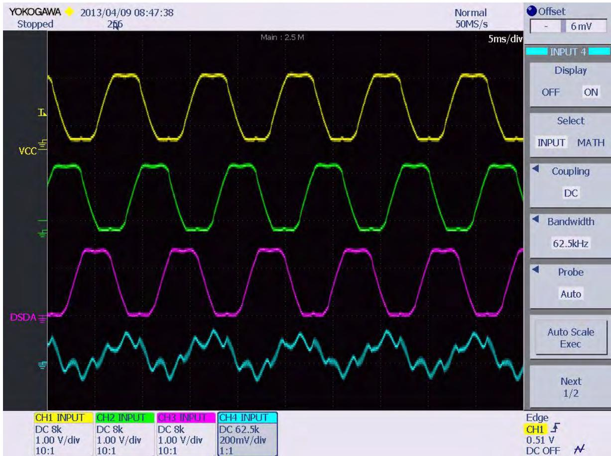
Figure 7. Linux BLDC Motor Phase Voltages and One Current Waveform
