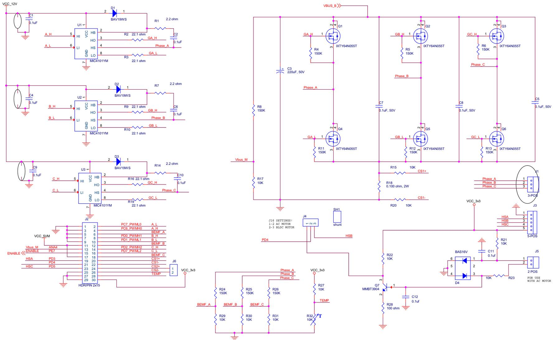
Figure 11. MultiMotor Development Board, #1 of 2
