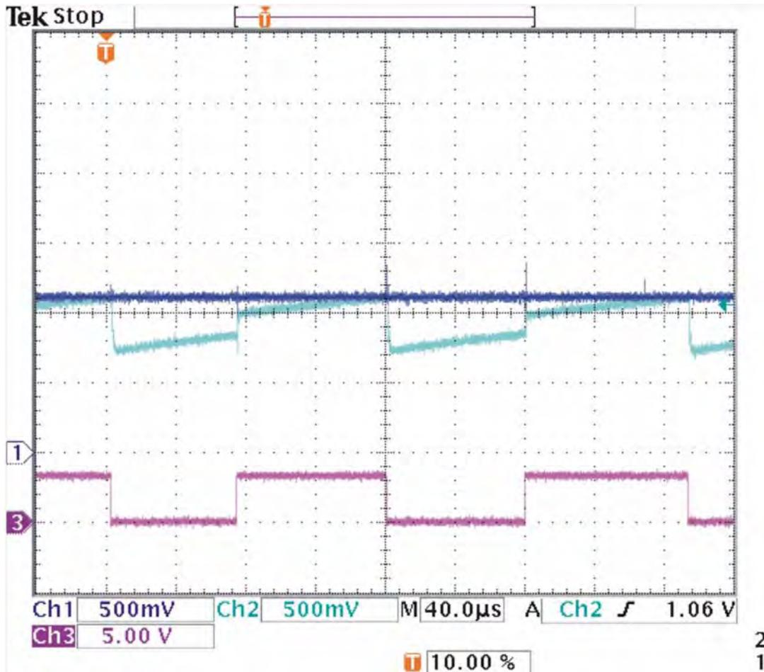
Figure 5. Cycle-by-Cycle Shutdown
