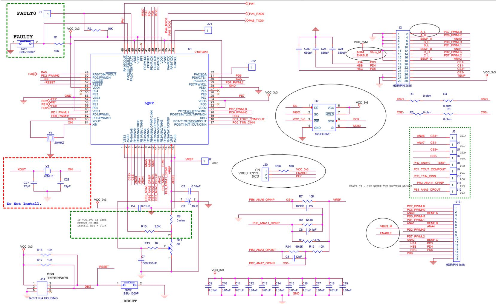
Figure 9. Z16FMC MultiMotor MCU Module, #1 of 2
