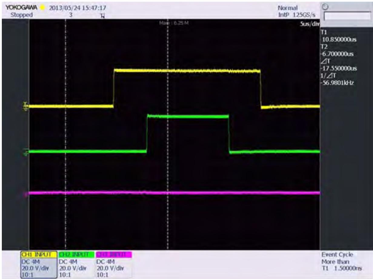
Figure 16.  $V_0$ ,  $V_7$  Space Vector Modulation Pattern
