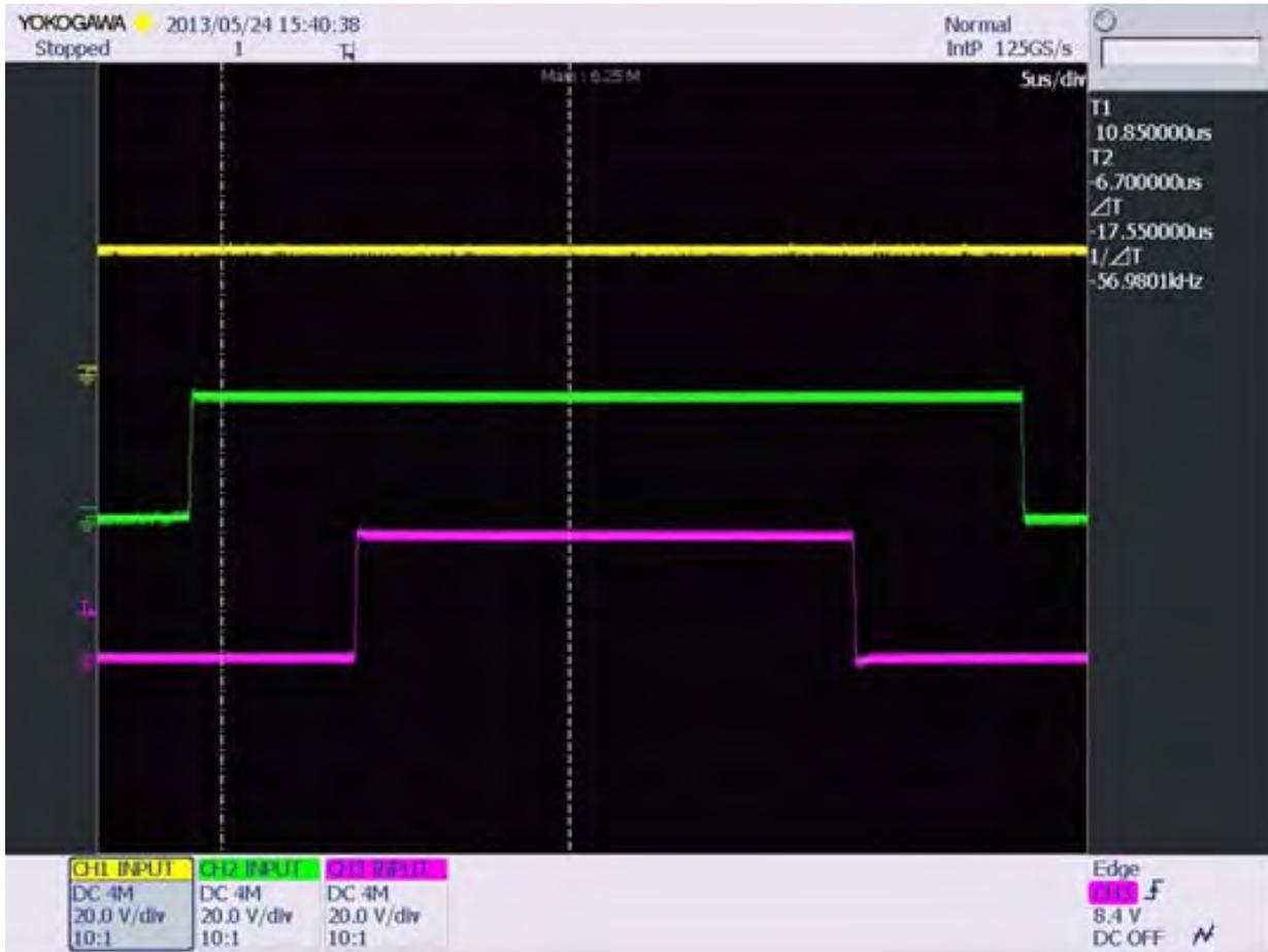
Figure 17.  $V_7$  Zero Vector Only Switching Pattern
