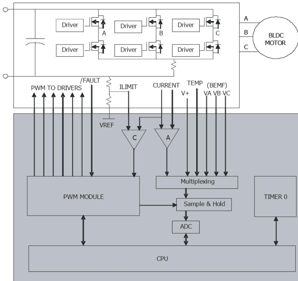
Figure 2. . A 3-Phase BLDC Motor Control System
