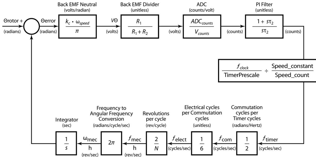
Figure 13. Back-EMF Sensing Using the Phase-Locked Loop Algorithm
