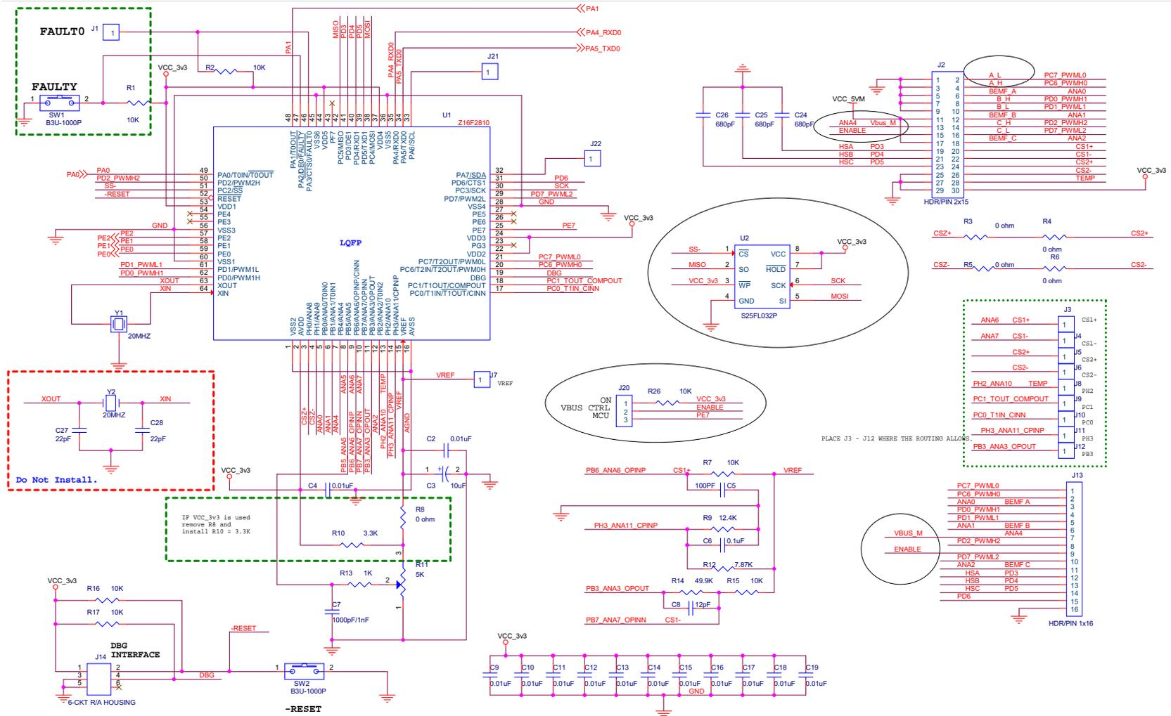
Figure 6. Z16FMC MultiMotor MCU Module, #1 of 2
