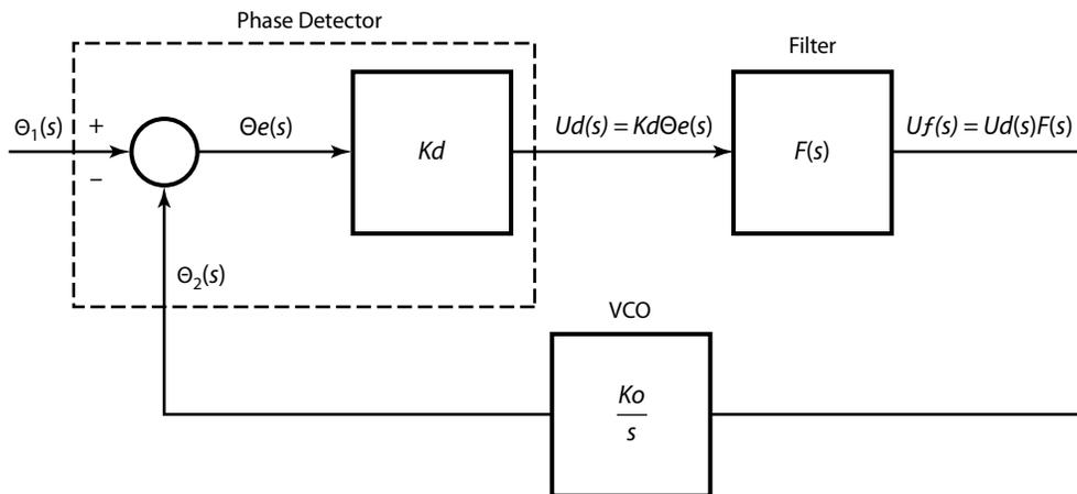
Figure 14. Proportional Integral (PI) Filter Representation for Back-EMF Sensing
