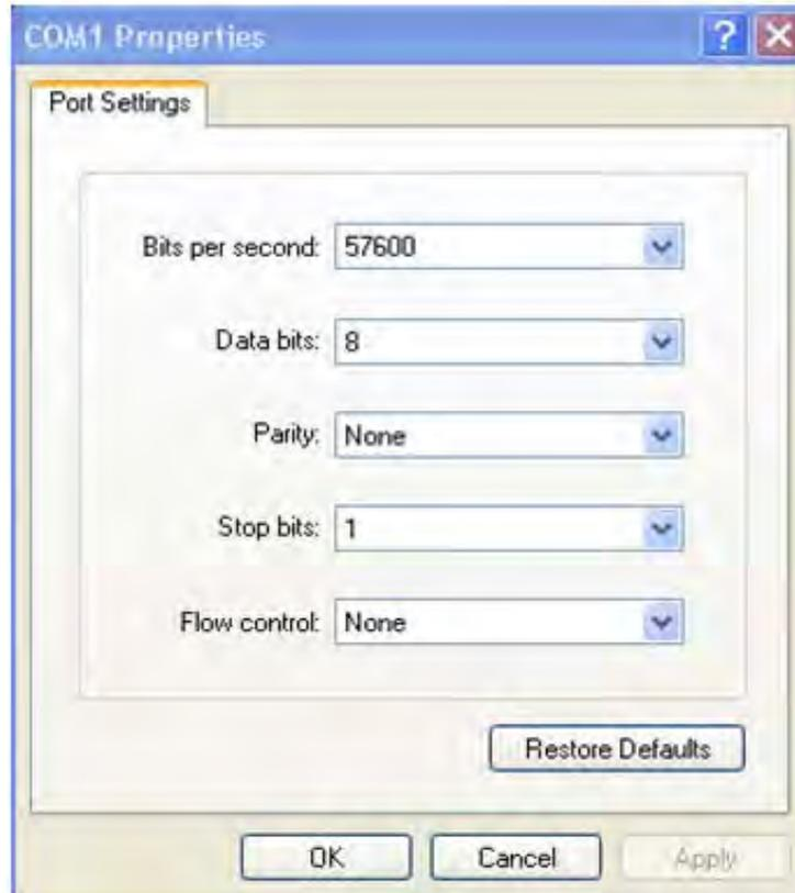
Figure 5. Example: Terminal Display Settings
