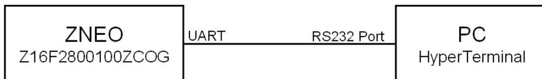
Figure 13. Z16FMC Series Development Kit to PC Connection via Serial (RS-232) Port
