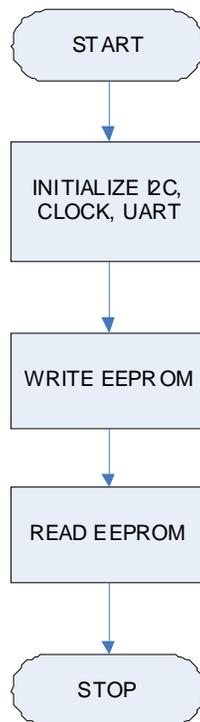
**Figure 38. I<sup>2</sup>C Main Function**
