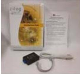
Zilog's S3 Flash ISP II provides an interface between any development or application board with an S3 microcontroller device to the high-speed USB port of a PC on which Zilog Developer Studio II for S3 Family devices (ZDS II – S3) is installed.
