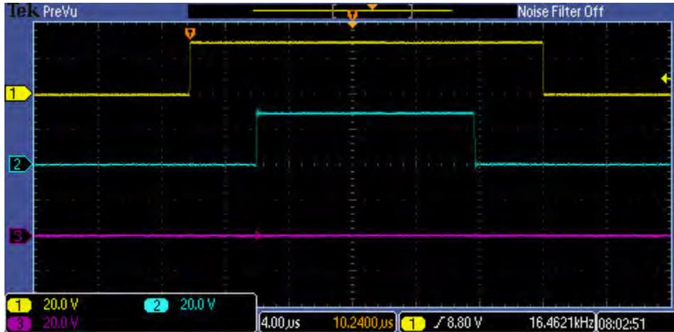
Figure 17. Alternate Switching Pattern at Time 3
