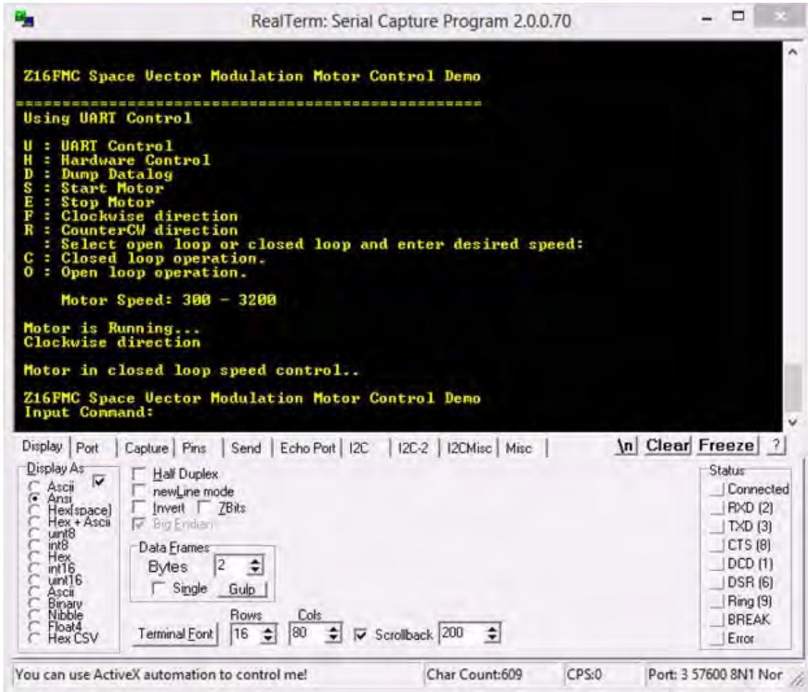
Figure 13. Console Display in UART Control Mode
