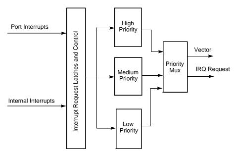
Figure 8. Interrupt Controller Block Diagram
