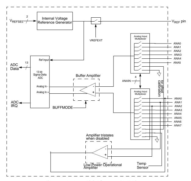
Figure 19. Analog-to-Digital Converter Block Diagram
