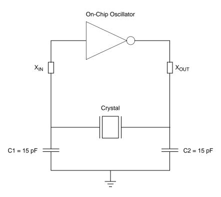
Figure 27. Recommended 20MHz Crystal Oscillator Configuration
