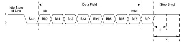
Figure 13. UART Asynchronous MULTIPROCESSOR Mode Data Format
