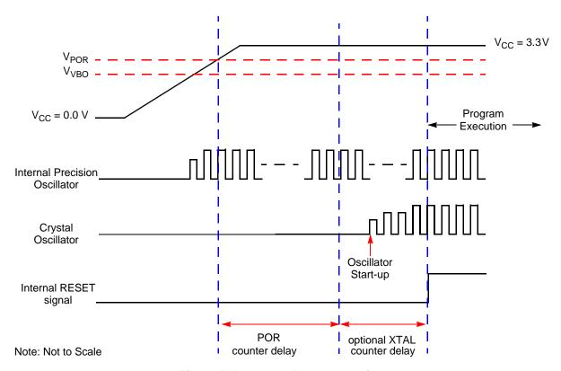
Figure 5. Power-On Reset Operation
