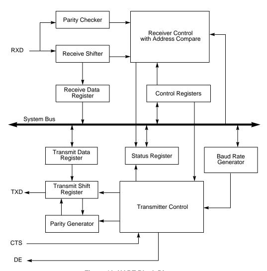
Figure 10. UART Block Diagram
