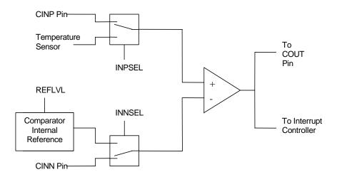
Figure 20. Comparator Block Diagram
