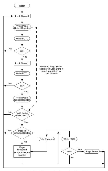
Figure 22. Flash Controller Operation Flow Chart
