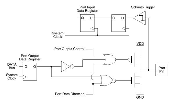
Figure 7. GPIO Port Pin Block Diagram
