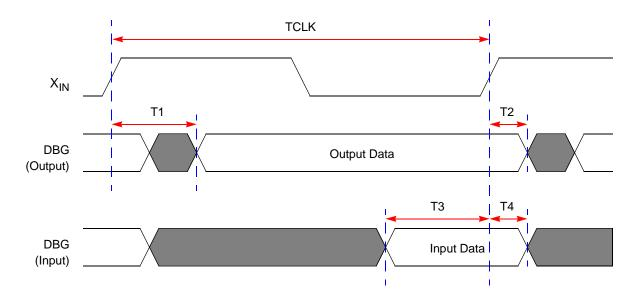
Figure 36. On-Chip Debugger Timing
