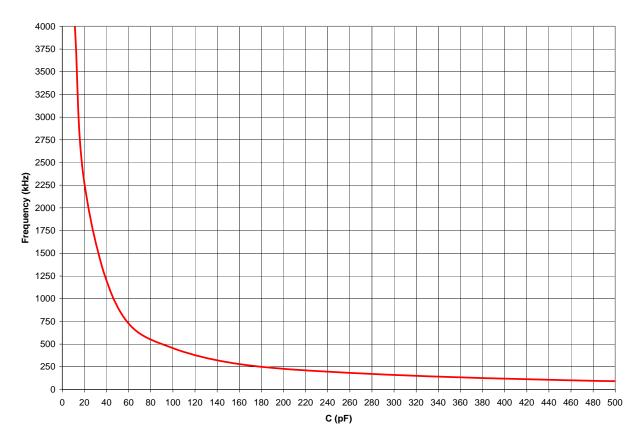
Figure 29. Typical RC Oscillator Frequency as a Function of the External Capacitance with a  $45k\Omega$  Resistor
