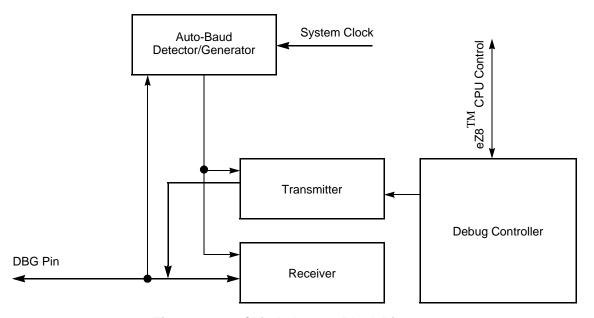
Figure 23. On-Chip Debugger Block Diagram
