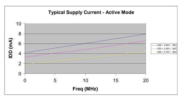
Figure 33. Typical Active Mode  $I_{DD}$  Versus System Clock Frequency
