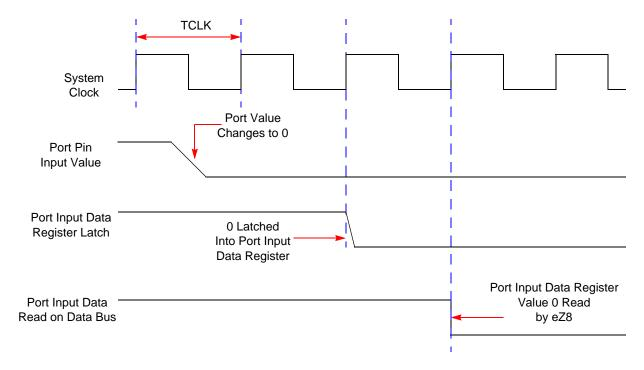
Figure 34. Port Input Sample Timing
