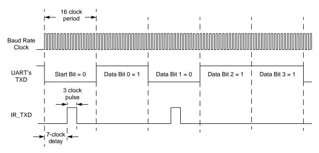
Figure 17. Infrared Data Transmission
