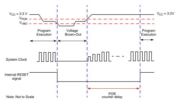
Figure 6. Voltage Brown-Out Reset Operation
