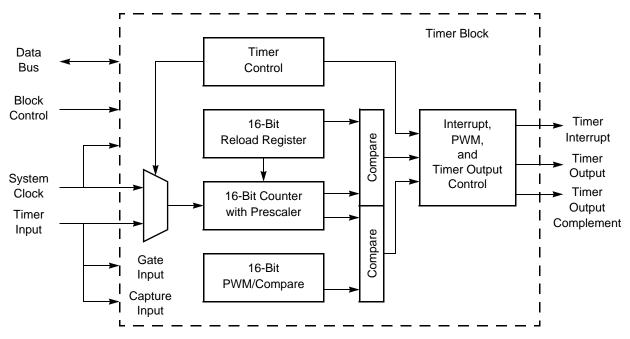
Figure 9. Timer Block Diagram
