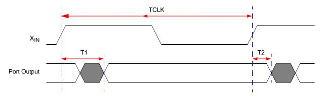
Figure 35. GPIO Port Output Timing
