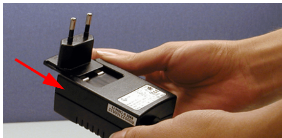
Figure 4. Inserting a New Plug Configuration
