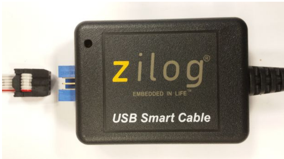
Figure 2. Connecting the 6-Circuit Ribbon Cable to the USB SmartCable
