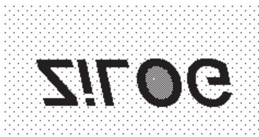
Figure 5. Snapshot of an Inverted BMP Image Displayed on a Graphic LCD
