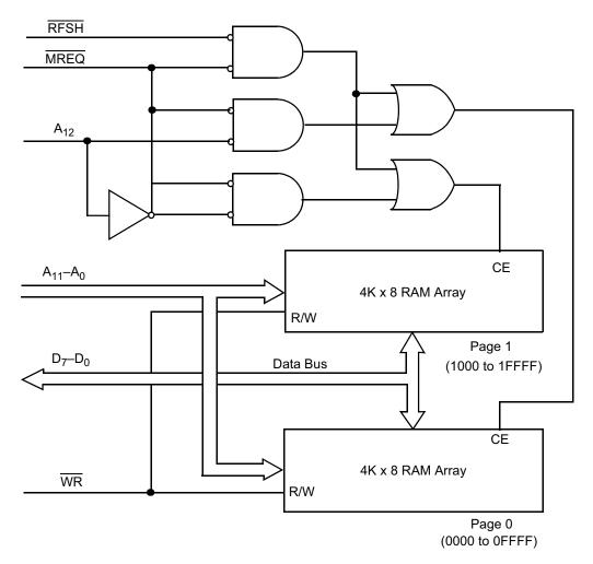
Figure 23. Interfacing Dynamic RAM Memory Spaces
