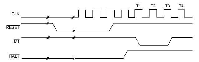
Figure 14. Power-Down Release Cycle, #2 of 3
