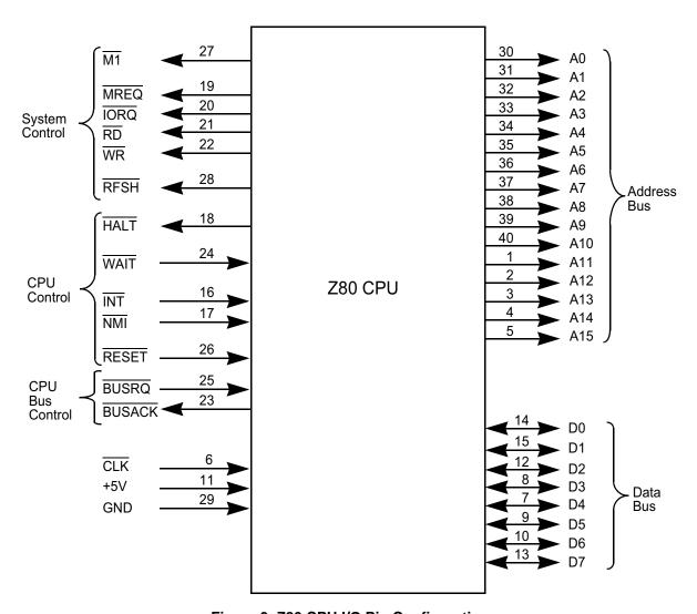
Figure 3. Z80 CPU I/O Pin Configuration
