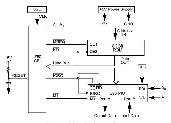
Figure 18. Minimum Z80 Computer System
