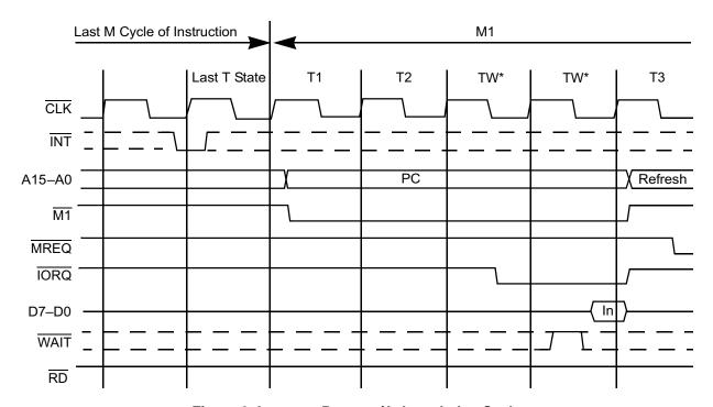
Figure 9. Interrupt Request/Acknowledge Cycle
