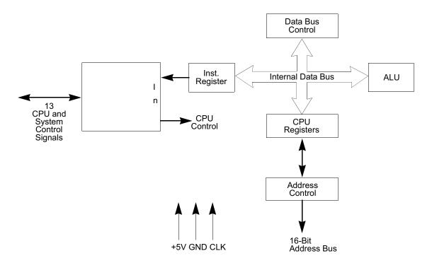
Figure 1. Z80 CPU Block Diagram
