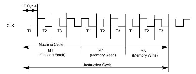
Figure 4. Basic CPU Timing Example
