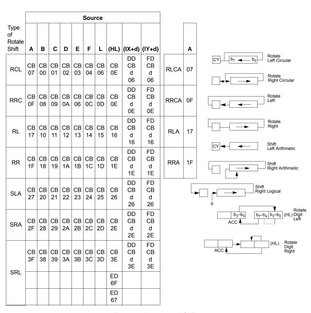
Figure 39. Rotates and Shifts
