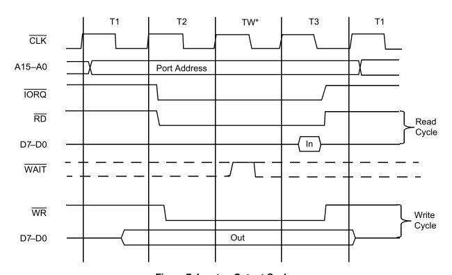
Figure 7. Input or Output Cycles
