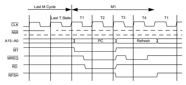
Figure 10. Nonmaskable Interrupt Request Operation
