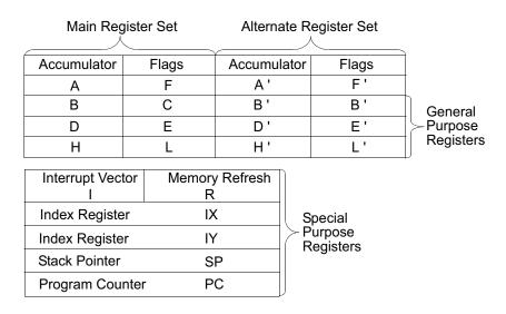
Figure 2. CPU Register Configuration
