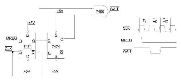
Figure 22. Adding One Wait State to Any Memory Cycle
