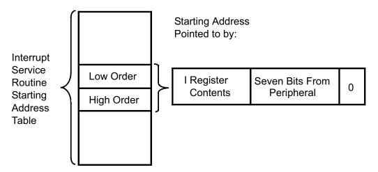
Figure 17. Mode 2 Interrupt Response Mode
