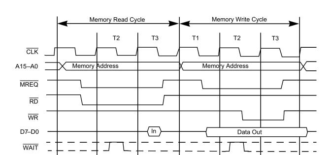
Figure 6. Memory Read or Write Cycle
