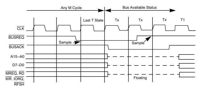
Figure 8. Bus Request/Acknowledge Cycle
