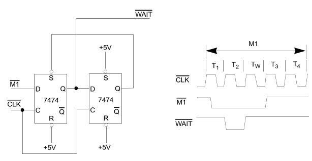
Figure 21. Adding One Wait State to an M1 Cycle
