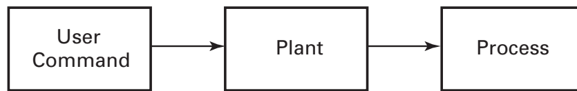
Figure 4. Block Diagram of an Open-Loop System
