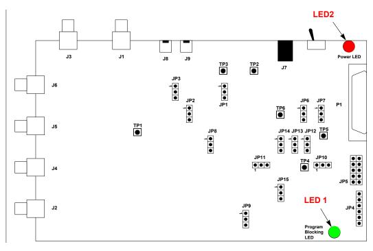
Figure 3. LEDs, Jumpers and Test Points
