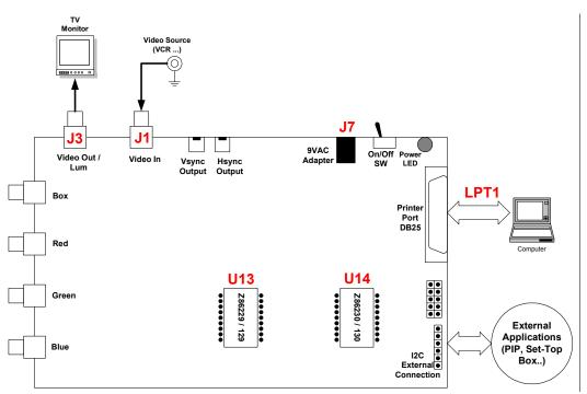
Figure 2. Demo Board System Configuration
