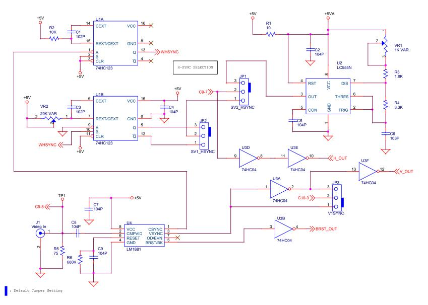
Figure 10. Video Front End Schematic
