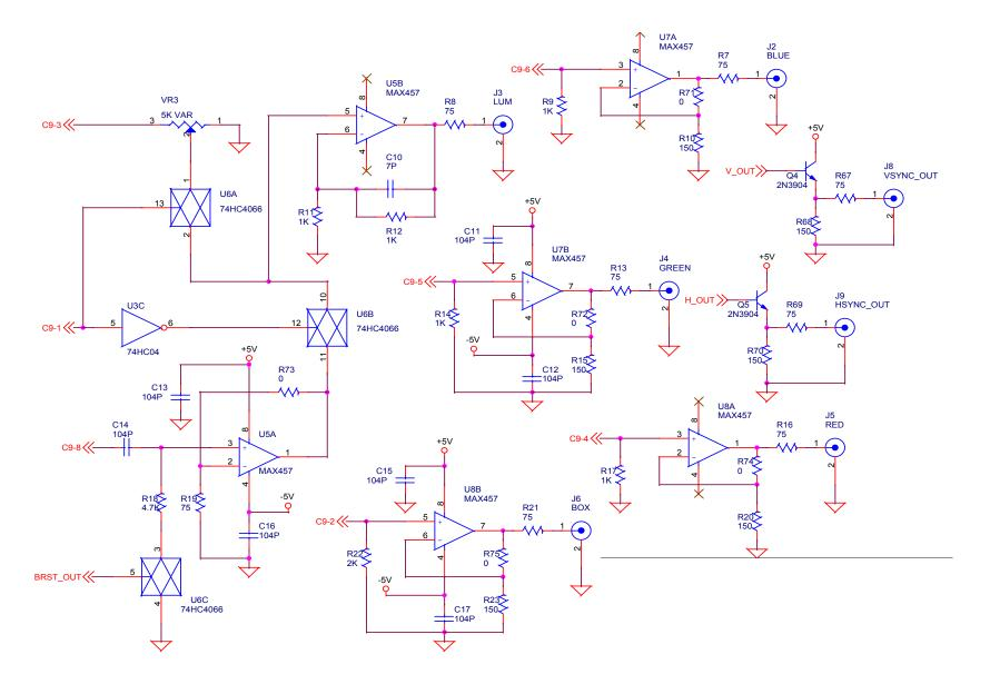
Figure 11. RGB Out Schematic
