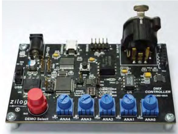
Figure 1. The DMX512-A Controller Reference Design
