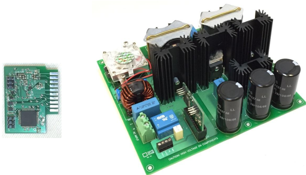
Figure 10. MCU Module (left) and Main Power Board with MCU Module (right)
