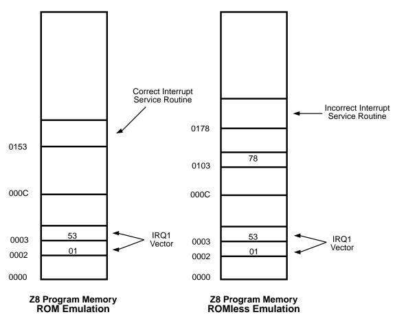
**Note:** The Incorrect Vectored Interrupt emulation only applies to the emulator. The Z89168/C68 device does not exhibit this problem.
