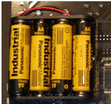
Figure 4. BT1 Battery Pack (Located on Back of MDS-GP Board)
