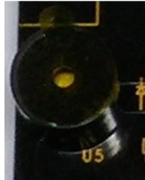
**Figure 15. Magnetic Buzzer**
