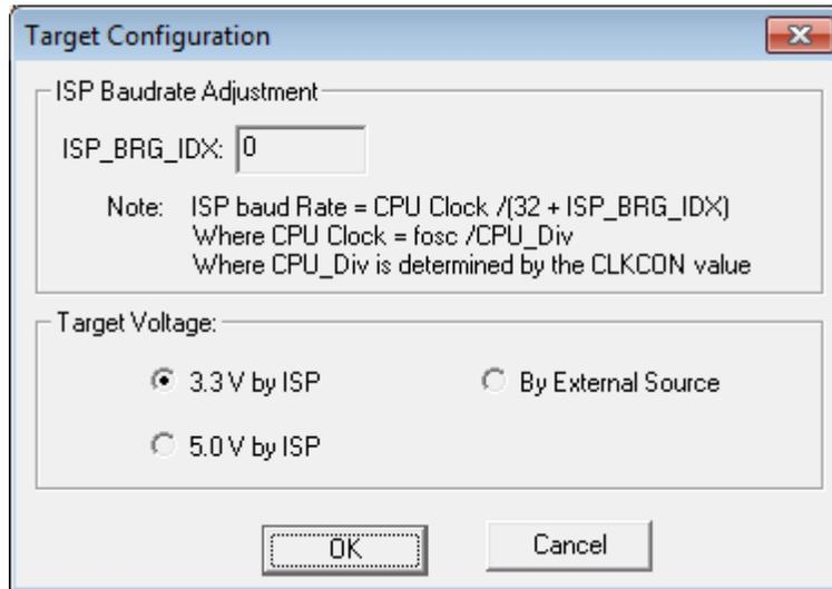
**Figure 10. The Target Configuration Dialog**
