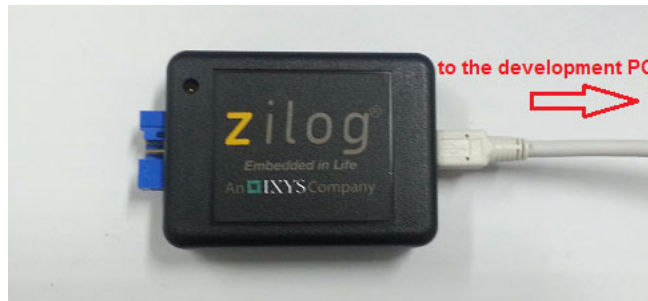
Figure 2. Connecting the S3 Flash ISP II to the Development PC
