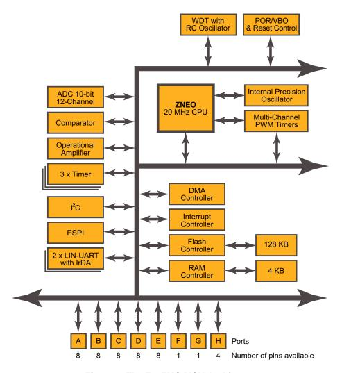
Figure 1. The Z16FMC MCU Architecture
