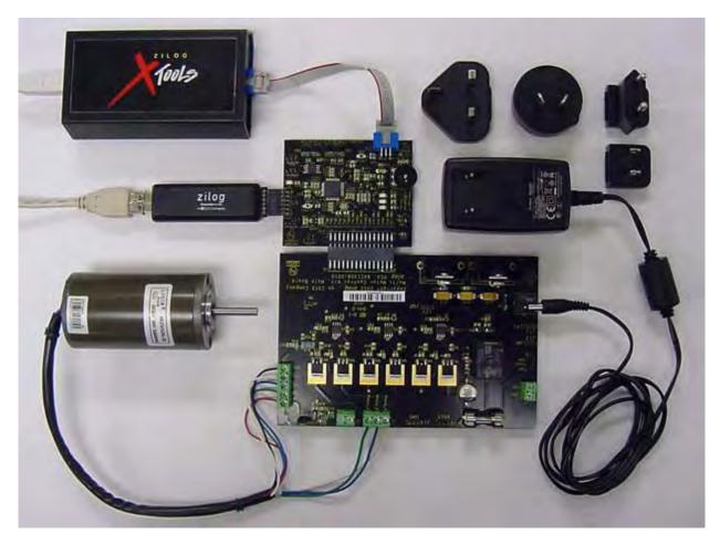
Figure 6. The MultiMotor Development Kit with Z16FMC MCU Module and SmartCable
