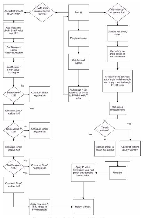
Figure 13. Simplified Control Algorithm
