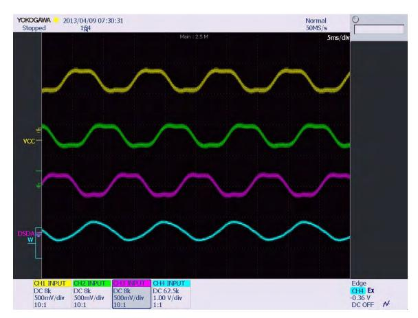
Figure 8. Linix BLDC Motor Phase Voltages and One Current Waveform
