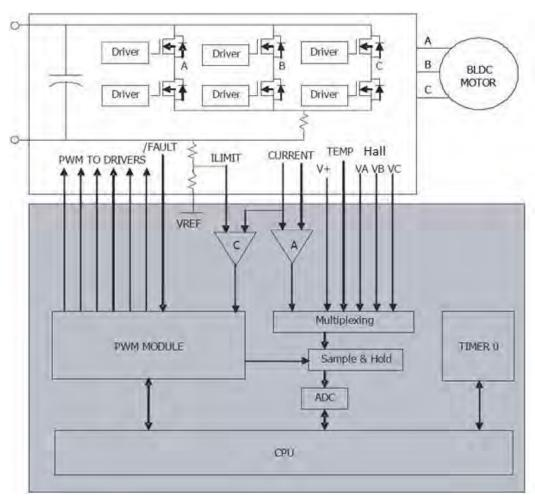
Figure 4. 3-Phase BLDC Motor Control System
