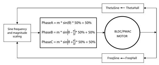
Figure 3. Simplified PWM Sine Operation of a BLDC Motor
