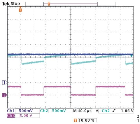
Figure 3. Cycle-By-Cycle Shutdown
