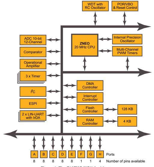
Figure 1. The Z16FMC MCU Architecture
