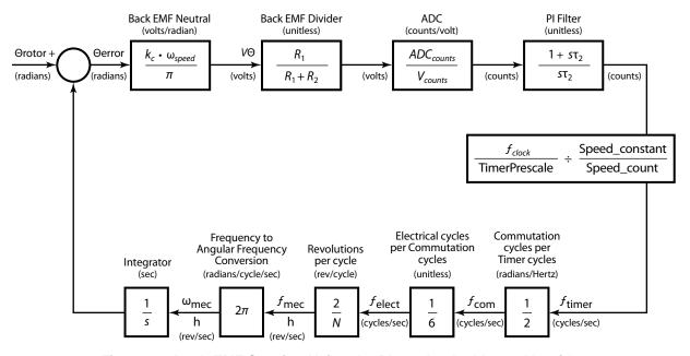
Figure 13. Back-EMF Sensing Using the Phase-Locked Loop Algorithm
