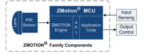
In addition to motion detection, the ZMOTION microcontroller can be used to perform additional functions such as input sensing, output control, and handling other tasks as required by the application.
