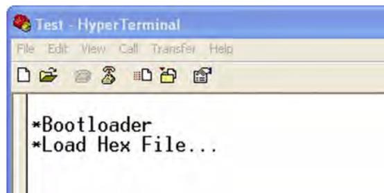
Figure 8. HyperTerminal Display After Boot Loader Initialization
